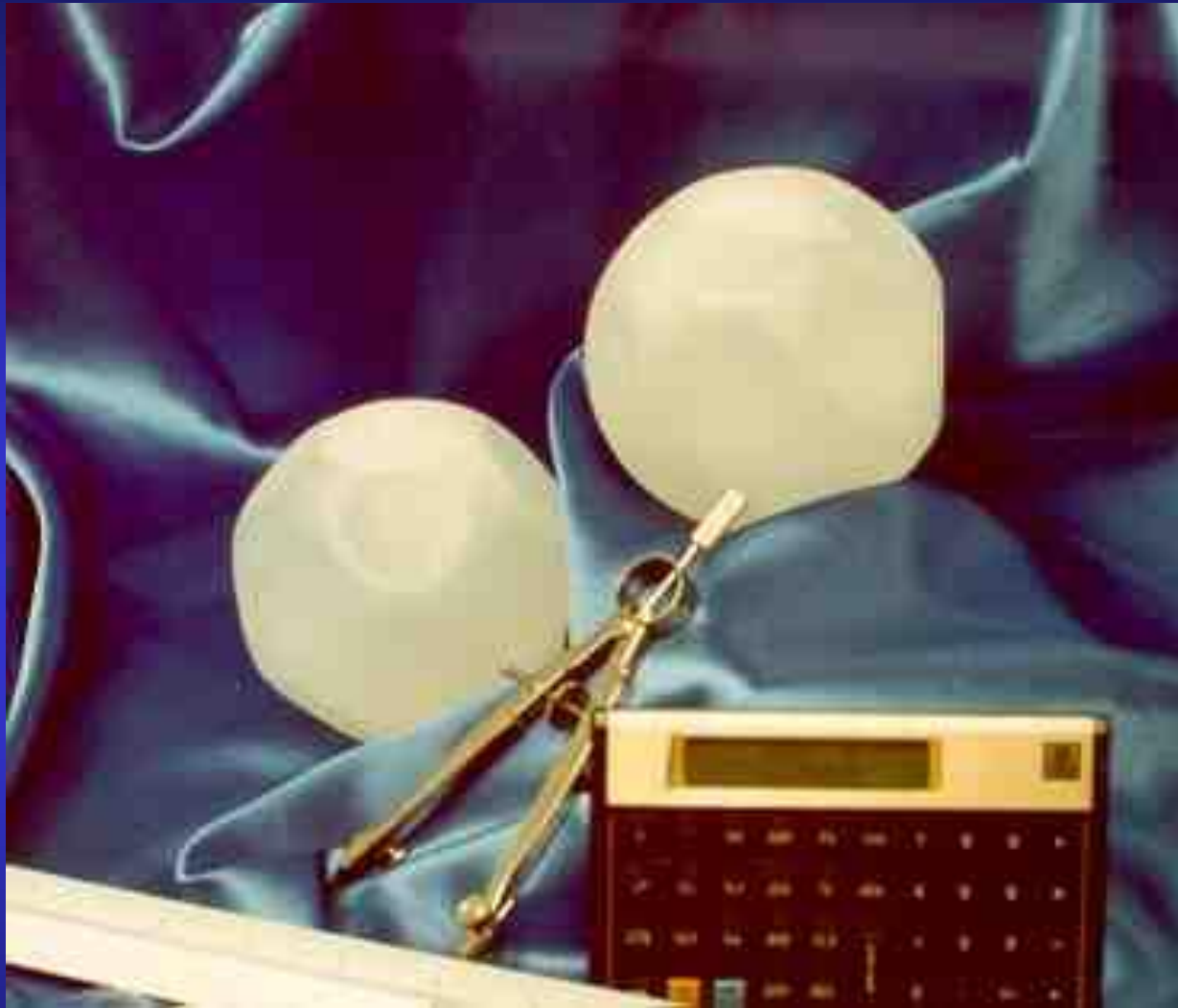
Ice Balls - Four Inch Diameter Plastic Spheres Filled With Water
